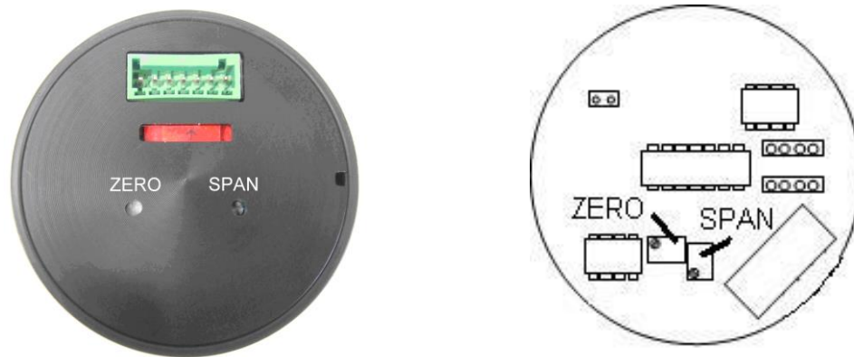
fig. 4.5.3.: Span adjust for different type of transmitter board.
